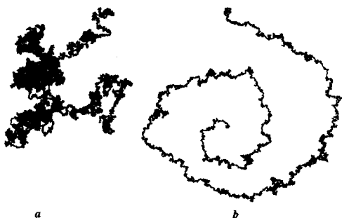
Fig. 6. a) A trace of 1.45 \times 10^5 random-walk steps. b) A trace of a spirally biased random walk ( 4.0 \times 10^4 steps). These are two paths from an external starting point to the growing seed.
